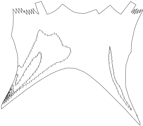
Fig. 2. Density profile of \text{He}^{2+} calculated with DORIS (in \text{m}^{-3} ).
