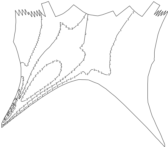
Fig. 3. Density profile of \text{He}^{2+} calculated with B2 (in \text{m}^{-3} ).
